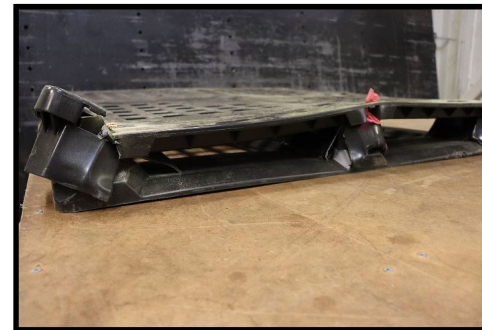
Damage after Hot Repetitive Shock
