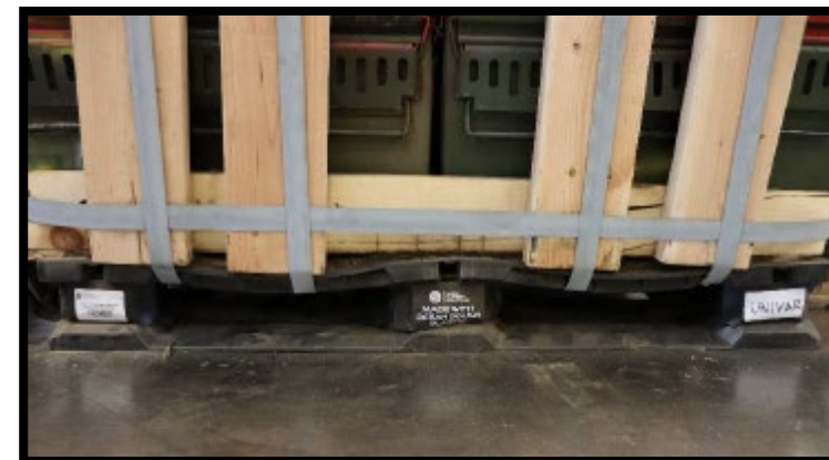
Visible Sagging after 4000 Hot Temperature Edgewise Drops
